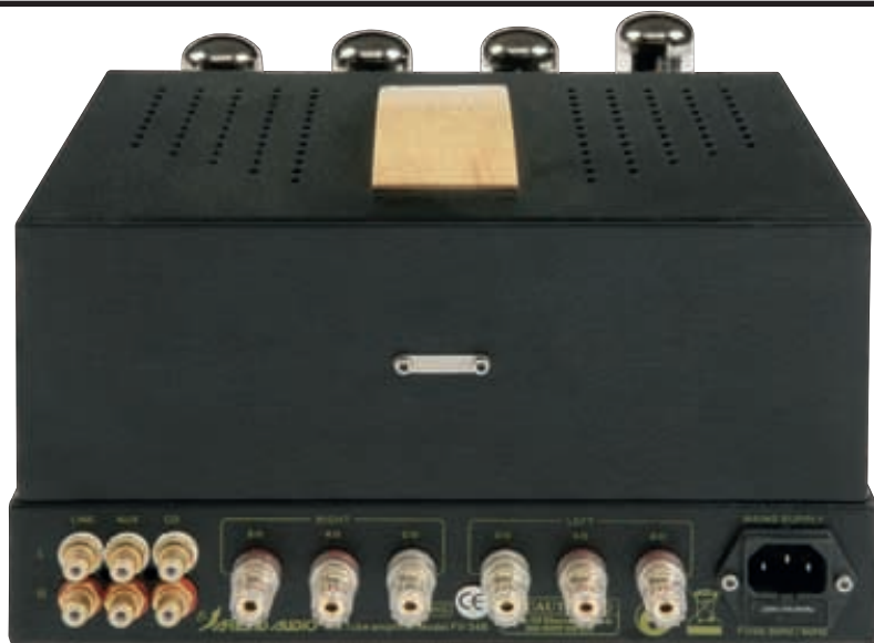
ABOVE: RCA sockets for three line inputs are included alongside separate 8ohm and 4ohm loudspeaker taps in the form of chunky 4mm binding posts
